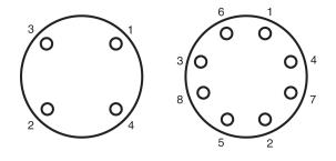
NOTE: USE WELL LUBRICATED METAL BOLTS AND NUTS. USE SOFT RUBBER GASKETS. NOTE: DUE TO THE DESIGN OF THE VG SERIES DIAPHRAGM VALVES, SIMTECH RECOMENDS THE USE OF LOW PROFILE NUT(JAM NUTS)
