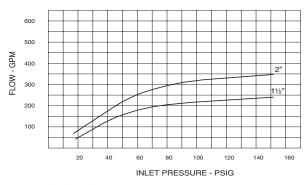
The performance curves are showing the flow rate of RBP with its piston seals is fully open, and 100% of the fluid flow thru the valve. These curves will be changed depend upon to the flow of the system and at each different pressure setting point.
