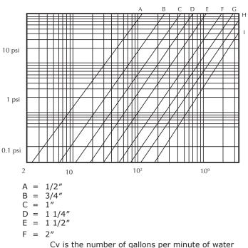
Cv is the number of gallons per minute of water at a temperature of 68°F that will flow through a valve with a 1 psi pressure differential at a specified travel.
