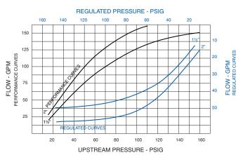
Performance curves show the flow rate of DPR valves with piston seal fully open. Regulated curves show the flow rate of DPR valves at the points of pre-set downstream pressure. Test data was performed with 68°F water, and 160 psig maximum pressure.
